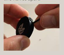
1.5. Remove the old battery by sliding it out of the metal cavity. To do this, you may need to lightly pull up on the small green electronic board so that you can slide out the old battery.
