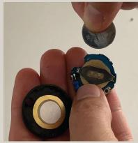
Insert the new battery with the + side facing up.
